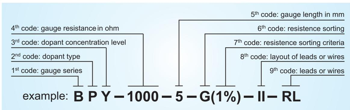
**1<sup>st</sup> code: gauge series** – whether the gauge is with or without the backing layer.
