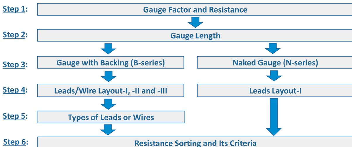
**Step 1:** Decide the gauge factor and resistance by considering the electronics of the data acquisition circuitry or system.
