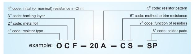
1st code: resistor type – whether the grid of the resistor is encapsulated or not.
